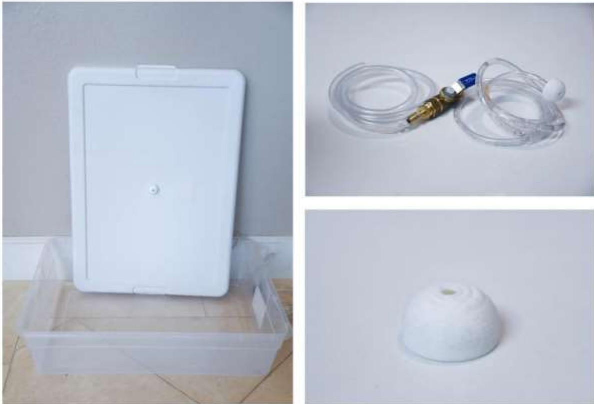
Supplementary Figure 4 | Mock ostomy setup. The setup included a plastic box with a lid drilled with a 1/4 th inch hole in the center to allow plastic tubing to be thread through. The plastic tubing has a ball valve to regulate the amount of liquid flowing through the tube. The tube attaches to the 3D printed stoma part where water can flow out of the hole of the stoma.
