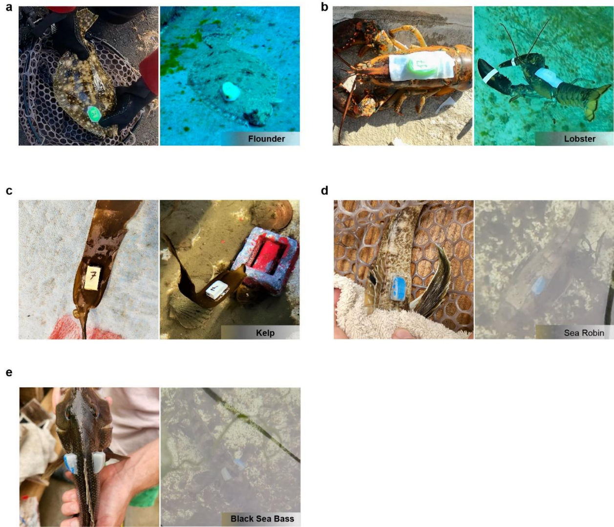
Supplementary Fig. 6 | Images and adhesion time for various marine species. a-e, Images of the BIMS applied to flounder, lobster, kelp, sea robin and sea bass before (left) and after (right) returning to the water.
